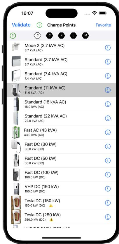
For each type of charging point (12 predefined), the essential characteristics are displayed; power and type of current and a typical photo of such a charging point.
